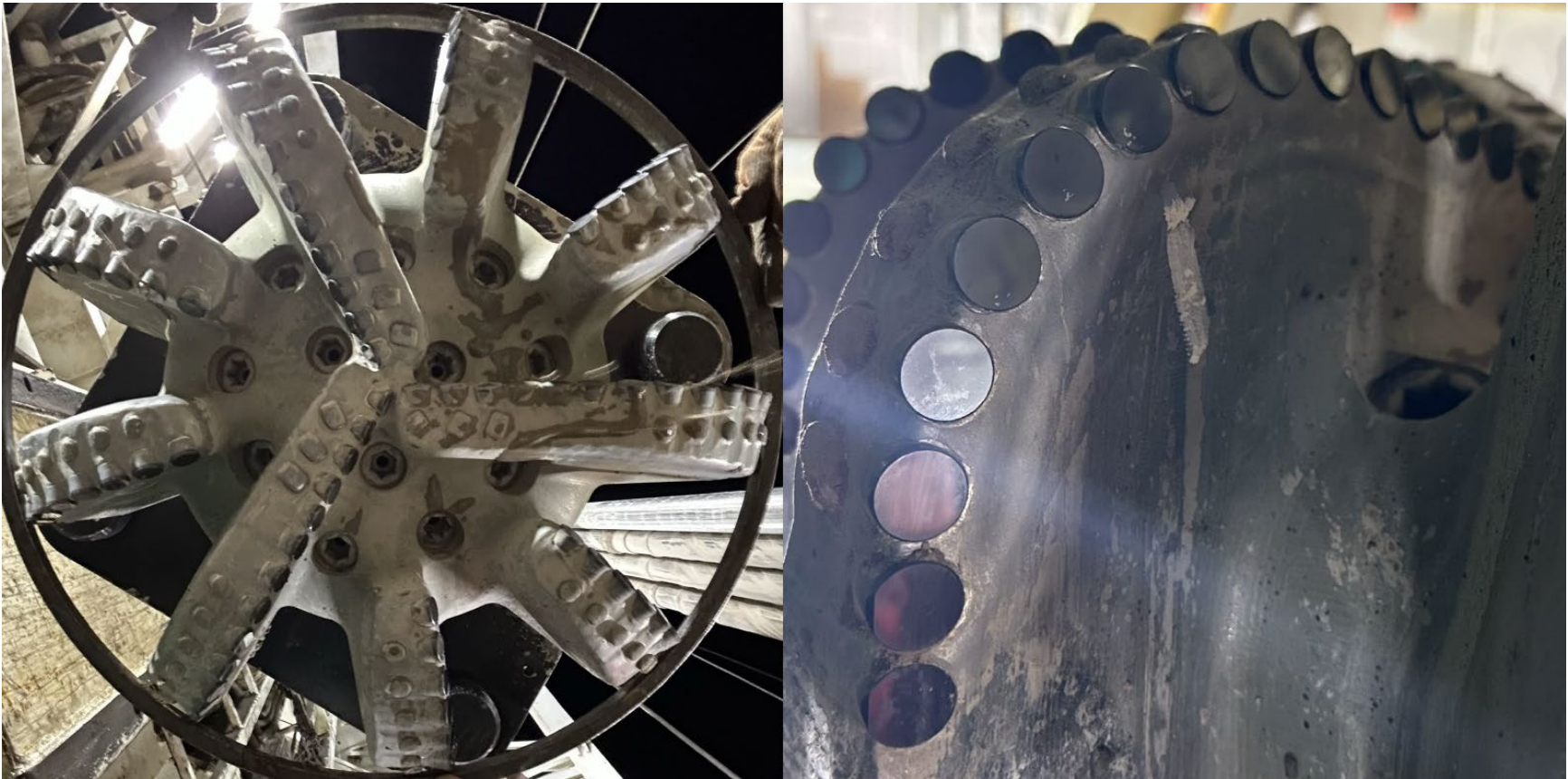
Figure 12. Dull photographs of the bit used for drilling the surface hole (BHA #1, TK99-A2).
