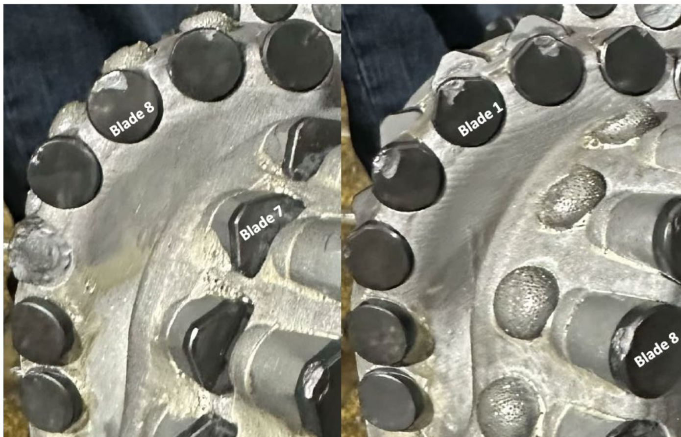
Figure 98. BHA #18 [9.5" TKC83-A2 (A298356)]. Compilation of dull photographs after drilling from 8,085 to 8,585 ft MD. Note - ReedHycalog and SDI refer to this as BHA #11 - it is in fact BHA #18. This was an NOV TKC83-A2 PDC bit. Pulled on schedule to test different bit performances.
