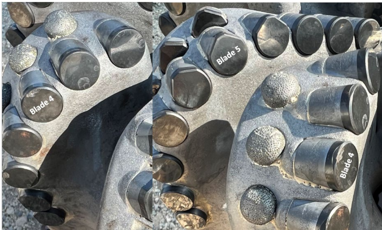
Figure 79. BHA #15 [9.5" TKC83-A2 (A298353)]. Compilation of dull photographs after drilling from 6,610 to 6,950 ft MD. Note - ReedHycalog and SDI refer to this as BHA #8 - it is in fact BHA #15. This was an NOV TKC83-A2 PDC bit. Pulled for logging after the build.
