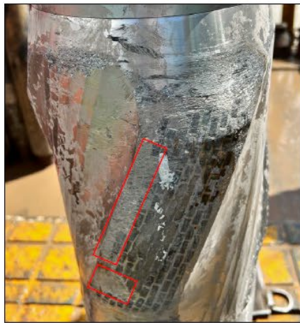
Figure F-3. Severe damage to the stabilizer and roller reamer.
