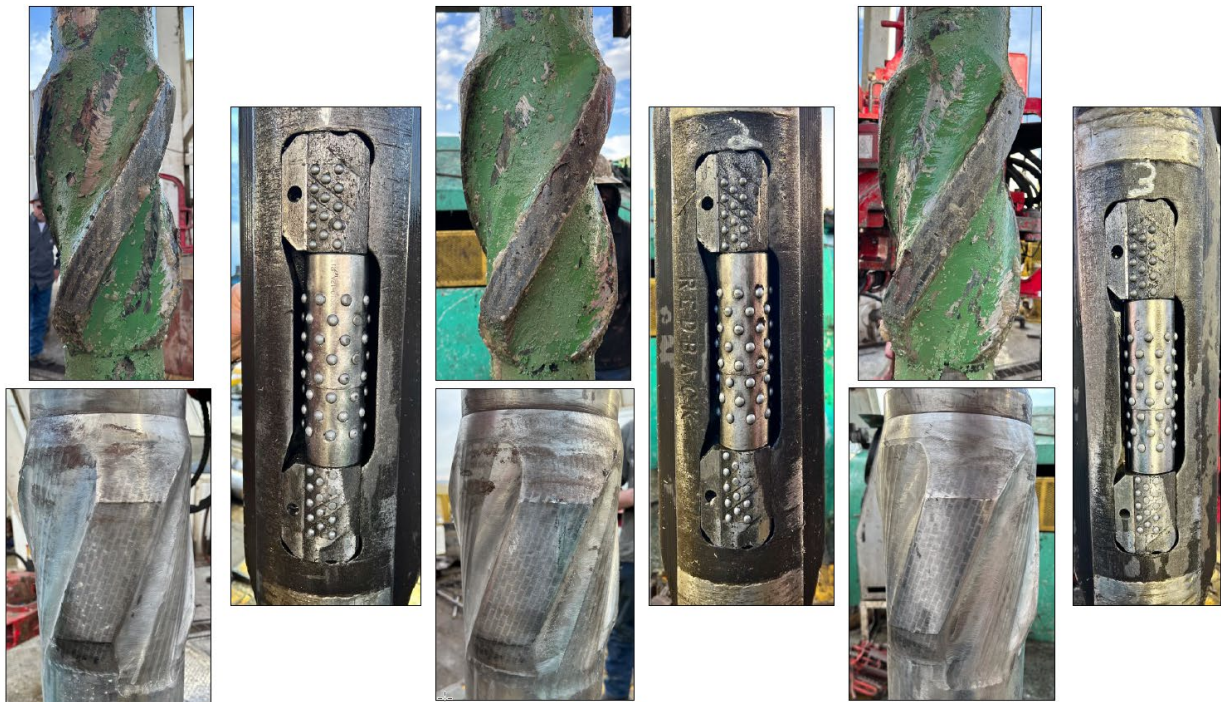
Figure F-32. The stabilizer and the roller reamer were pulled in good condition.
