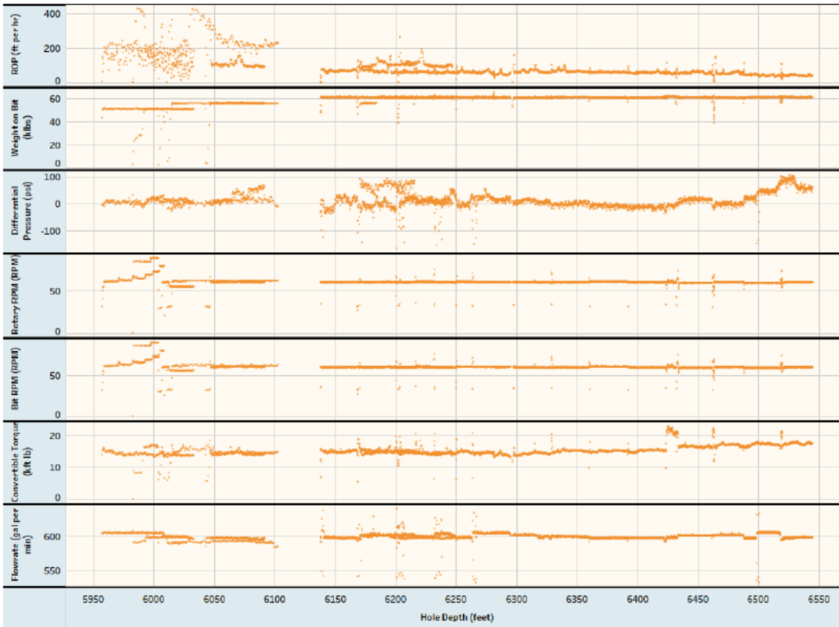
Figure 66. BHA #13 [9.5" TKC73-A2 (A298330)]. Compilation of drilling records for drilling from 5,957 to 6,545 ft MD. Note - ReedHycalog and SDI refer to this as BHA #6 - it is in fact BHA #13. This was an NOV TKC73-A2 PDC bit.
