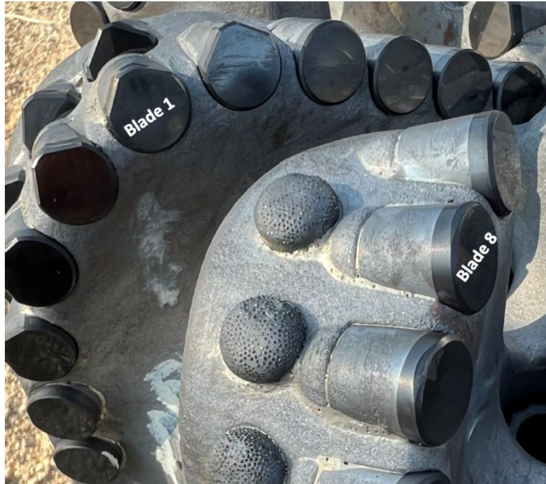
Figure 81. BHA #15 [9.5" TKC83-A2 (A298353)]. Compilation of dull photographs after drilling from 6,610 to 6,950 ft MD. Note - ReedHycalog and SDI refer to this as BHA #8 - it is in fact BHA #15. This was an NOV TKC83-A2 PDC bit. Pulled for logging after the build.
