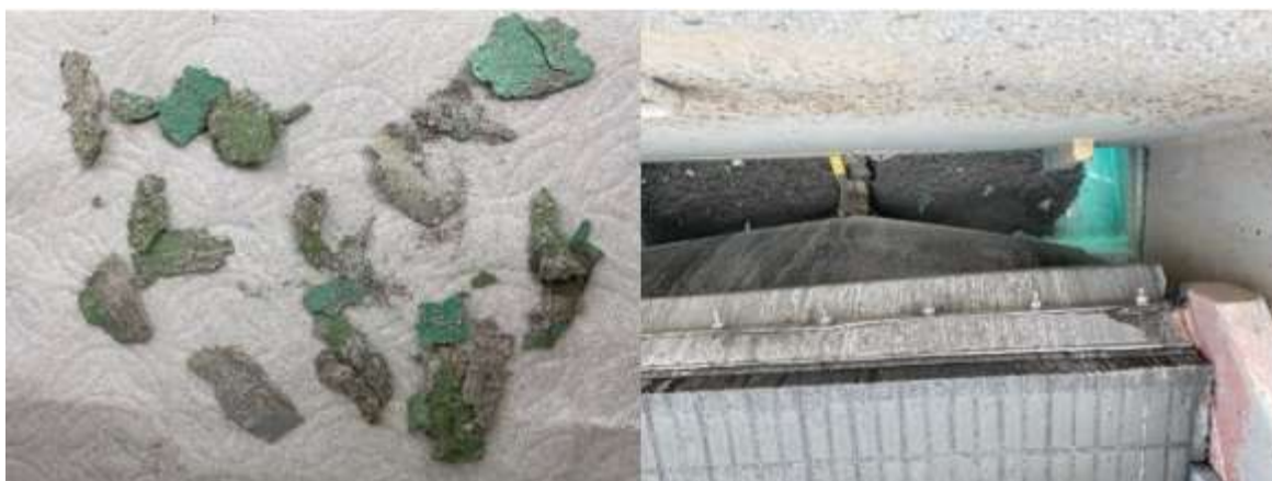
Figure D-7: Coating pieces caught by the mud loggers
