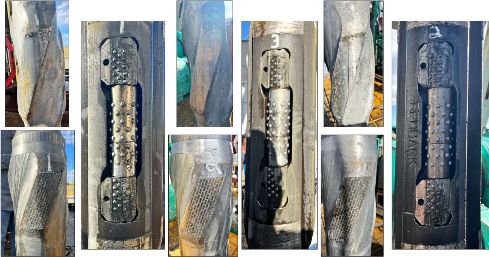
Figure F-13. The stabilizer and roller reamer were in good condition.
