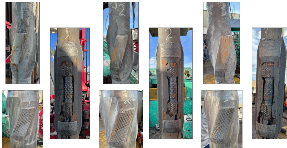
Figure F-21. Stabilizer and roller reamer were recovered in good condition.
