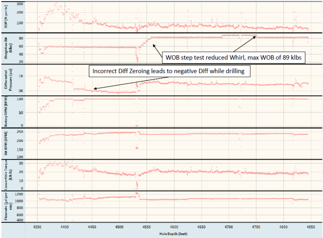
Figure 27. BHA #4 [14.75” TKC83-A2 (A298775)]. This bit drilled 492 ft in 7.2 hours at an average rate of penetration of 68 ft/hr. Note - ReedHycalog refers to this as BHA #3 - it is in fact BHA #4. This was an NOV TKC83-A2 PDC bit.
