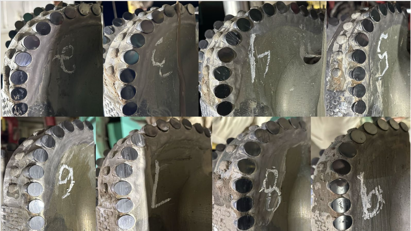
Figure 13. Dull photographs of the bit used for drilling the surface hole (BHA #1, TK99-A2).
