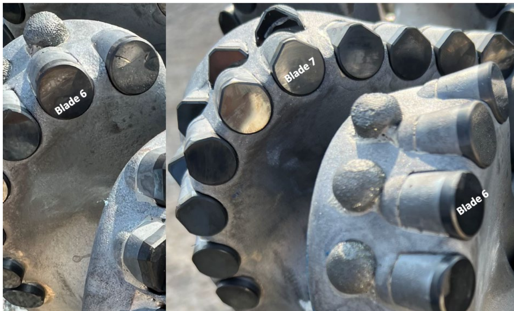
Figure 80. BHA #15 [9.5" TKC83-A2 (A298353)]. Compilation of dull photographs after drilling from 6,610 to 6,950 ft MD. Note - ReedHycalog and SDI refer to this as BHA #8 - it is in fact BHA #15. This was an NOV TKC83-A2 PDC bit. Pulled for logging after the build.
