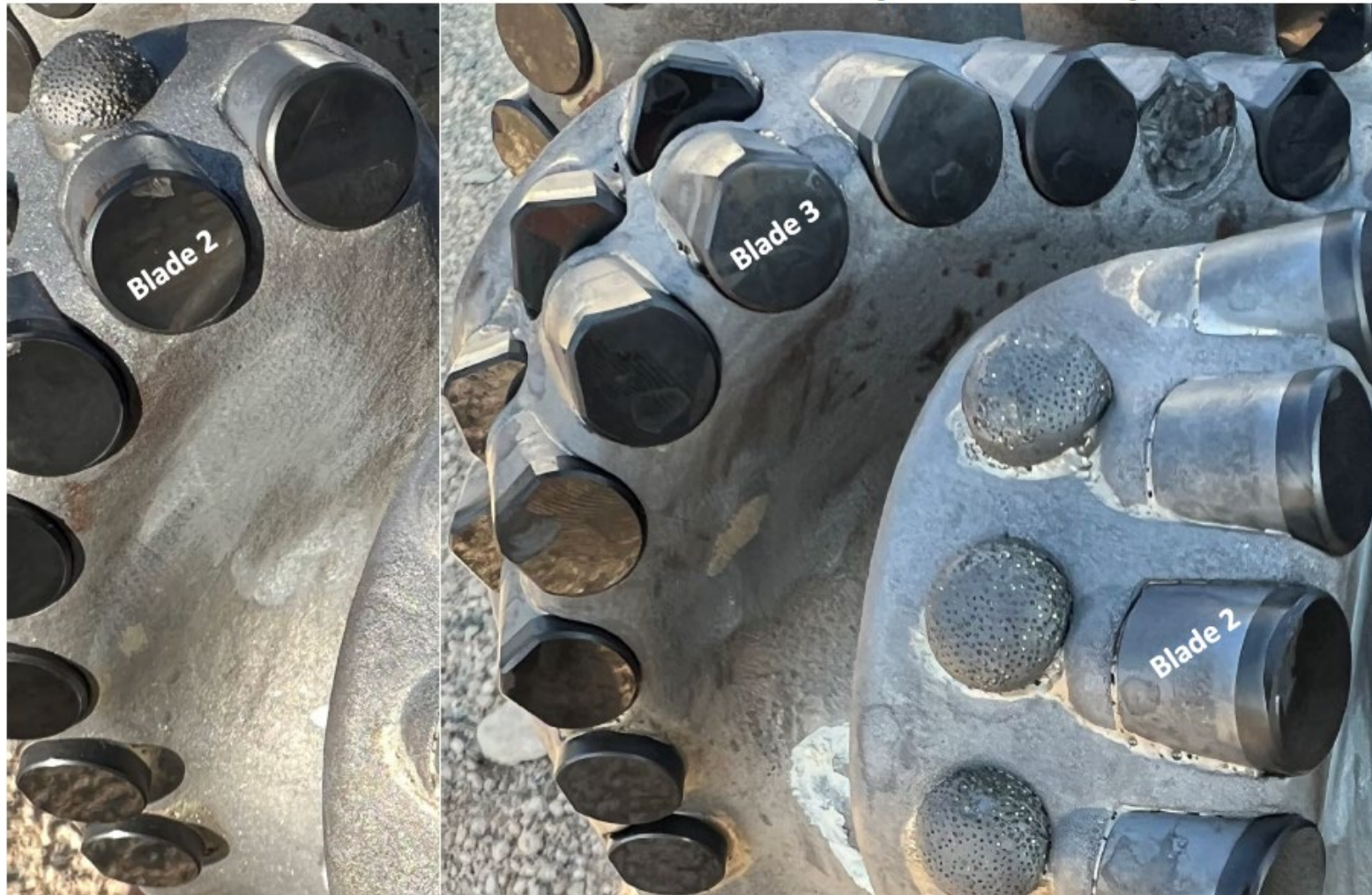
Figure 78. BHA #15 [9.5" TKC83-A2 (A298353)]. Compilation of dull photographs after drilling from 6,610 to 6,950 ft MD. Note - ReedHycalog and SDI refer to this as BHA #8 - it is in fact BHA #15. This was an NOV TKC83-A2 PDC bit. Pulled for logging after the build.
