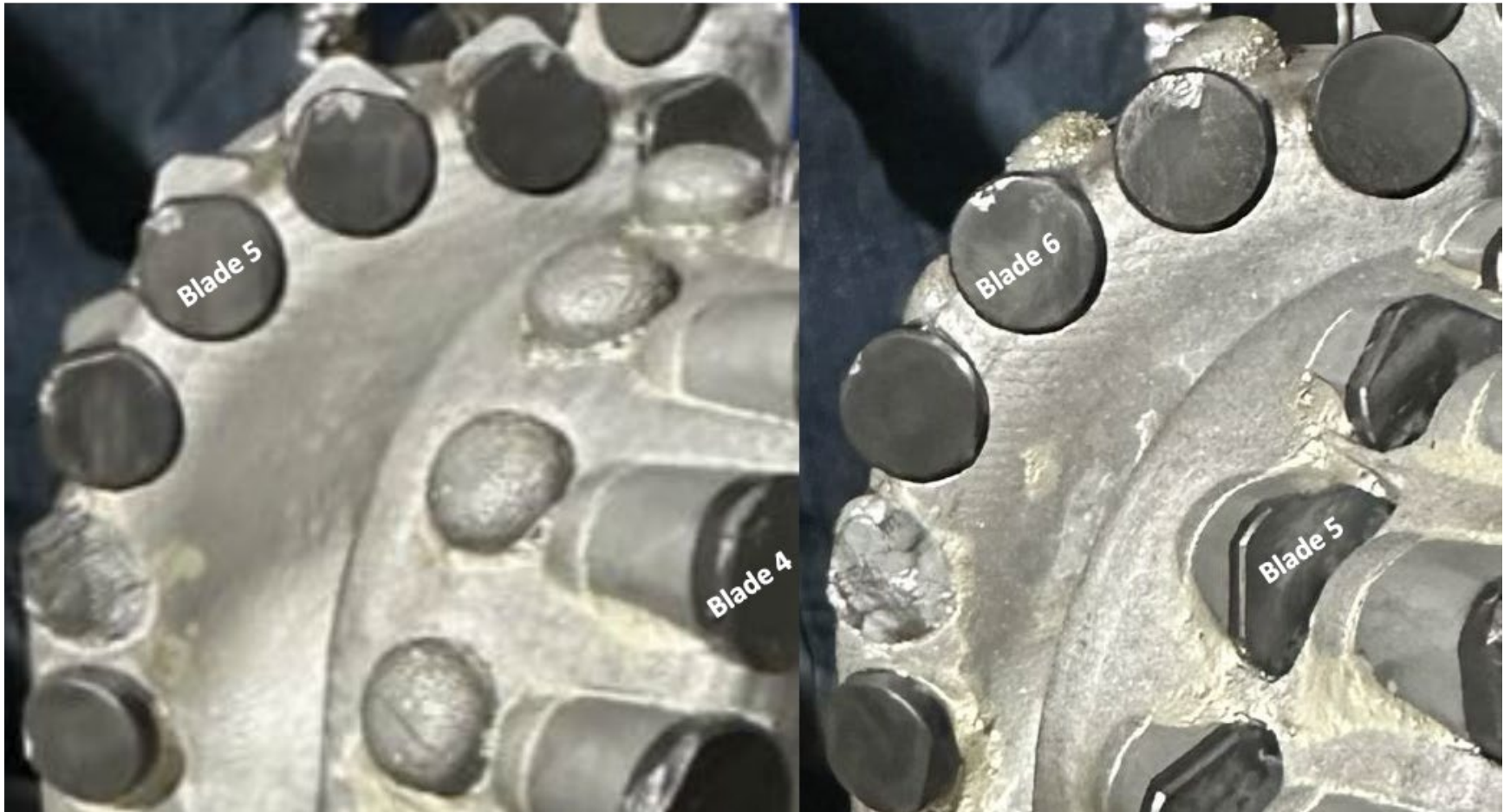
Figure 96. BHA #18 [9.5" TKC83-A2 (A298356)]. Compilation of dull photographs after drilling from 8,085 to 8,585 ft MD. Note - ReedHycalog and SDI refer to this as BHA #11 - it is in fact BHA #18. This was an NOV TKC83-A2 PDC bit. Pulled on schedule to test different bit performances.
