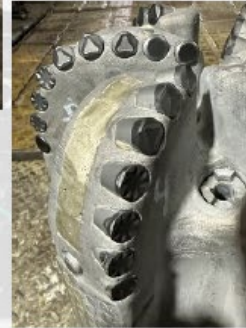
Cracked shoulder cutter
