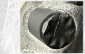
Cracked shoulder cutter
