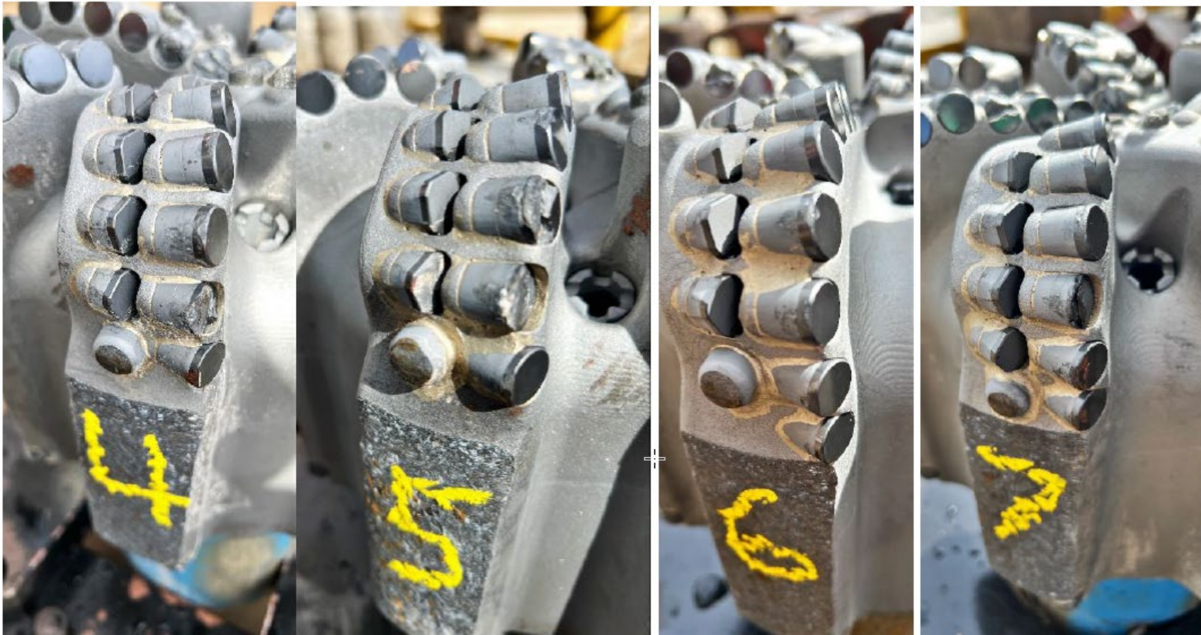
Figure 56. BHA #11 [9.5" TKC73-A2 (A298329)]. Compilation of bit dull photographs after drilling from 4,980 to 5,269 ft. Note - ReedHycalog refers to this as BHA #4 - it is in fact BHA #11. This was an NOV TKC73-A2 PDC bit. The BHA was pulled because of failure of the directional tools.
