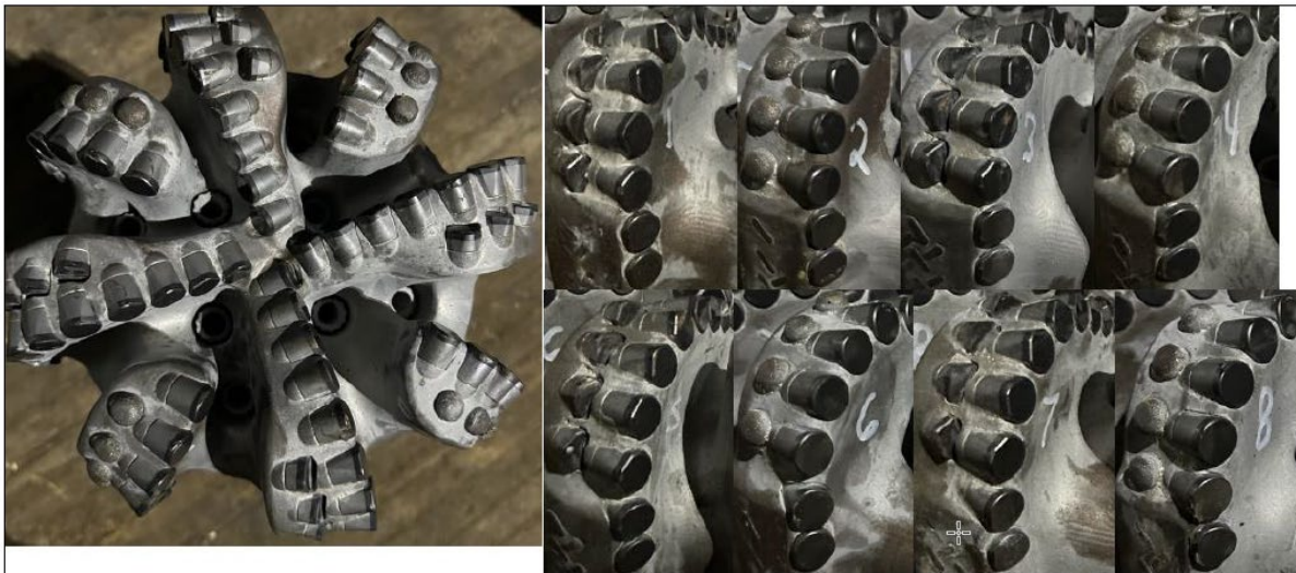
Figure F-49. Pulled bit (BHA 16).
