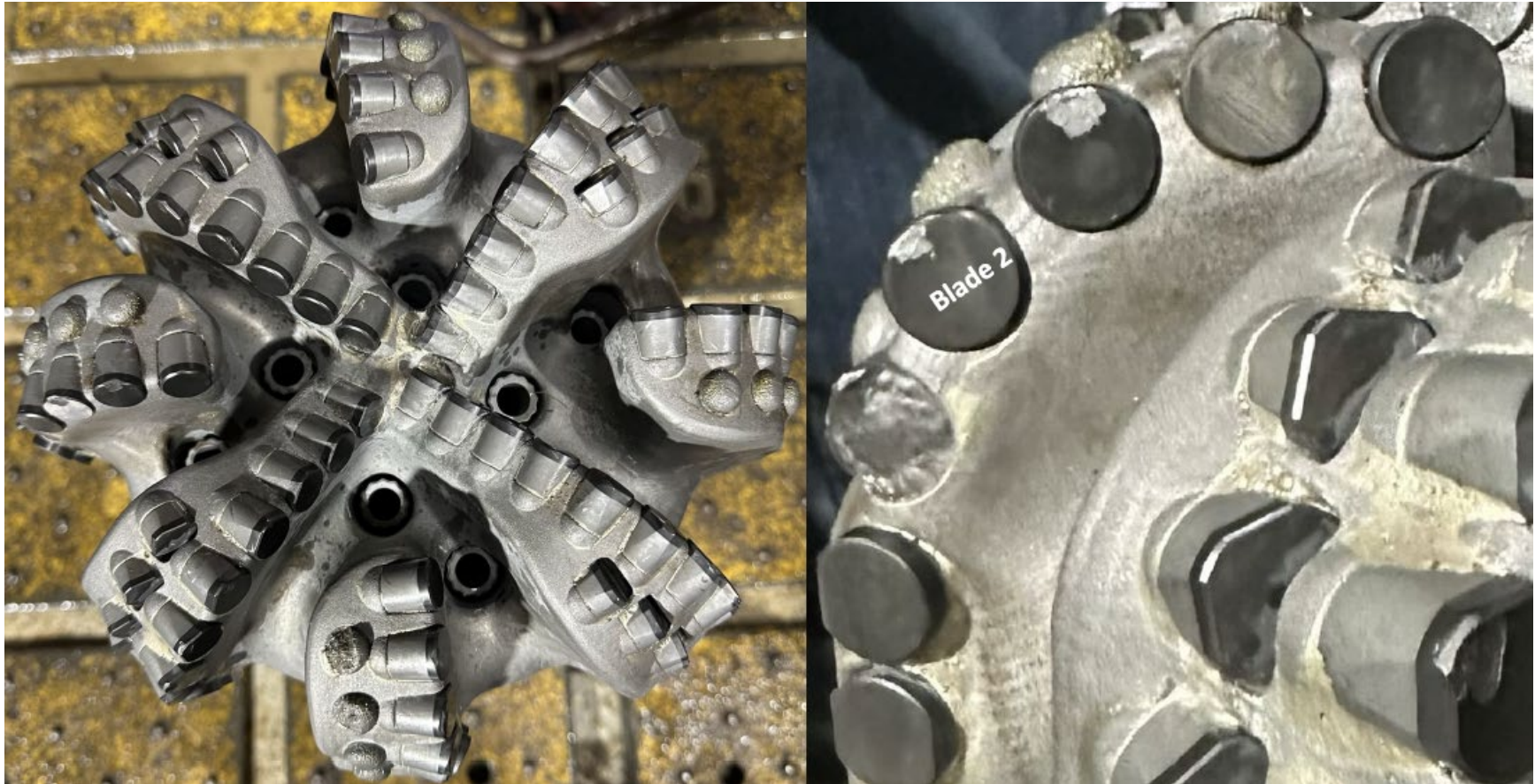
Figure 95. BHA #18 [9.5" TKC83-A2 (A298356)]. Compilation of dull photographs after drilling from 8,085 to 8,585 ft MD. Note - ReedHycalog and SDI refer to this as BHA #11 - it is in fact BHA #18. This was an NOV TKC83-A2 PDC bit. Pulled on schedule to test different bit performances.
