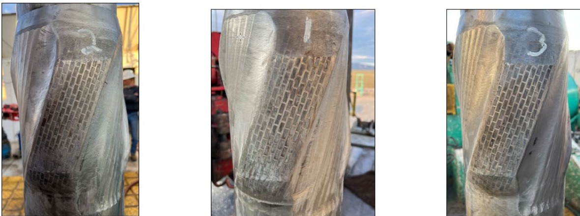
Figure F-40. Photographs of stabilizer (post-run).
