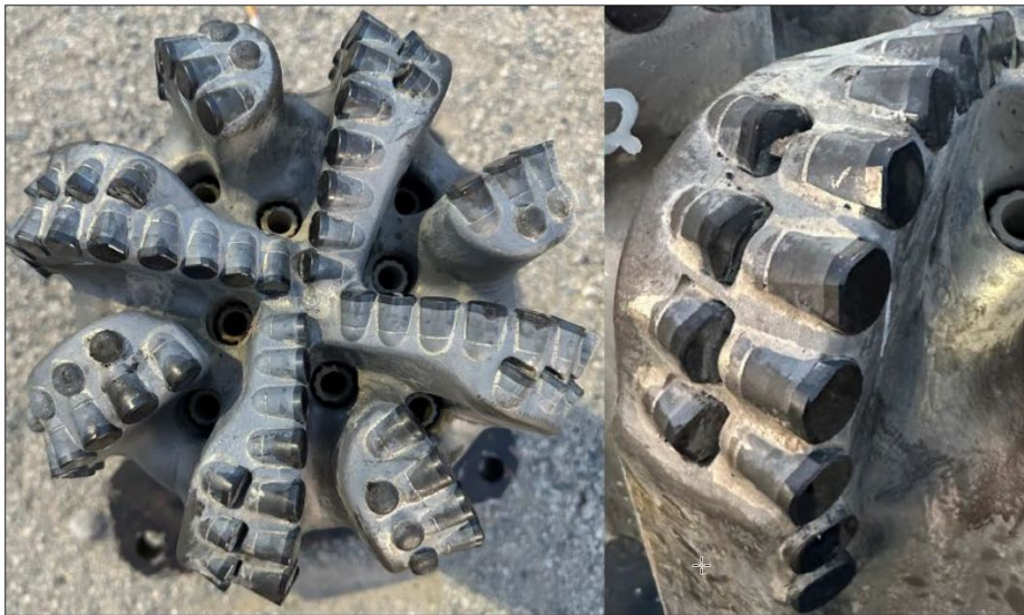
Figure F-31. Recovered bit was in good condition. This was a short run.
