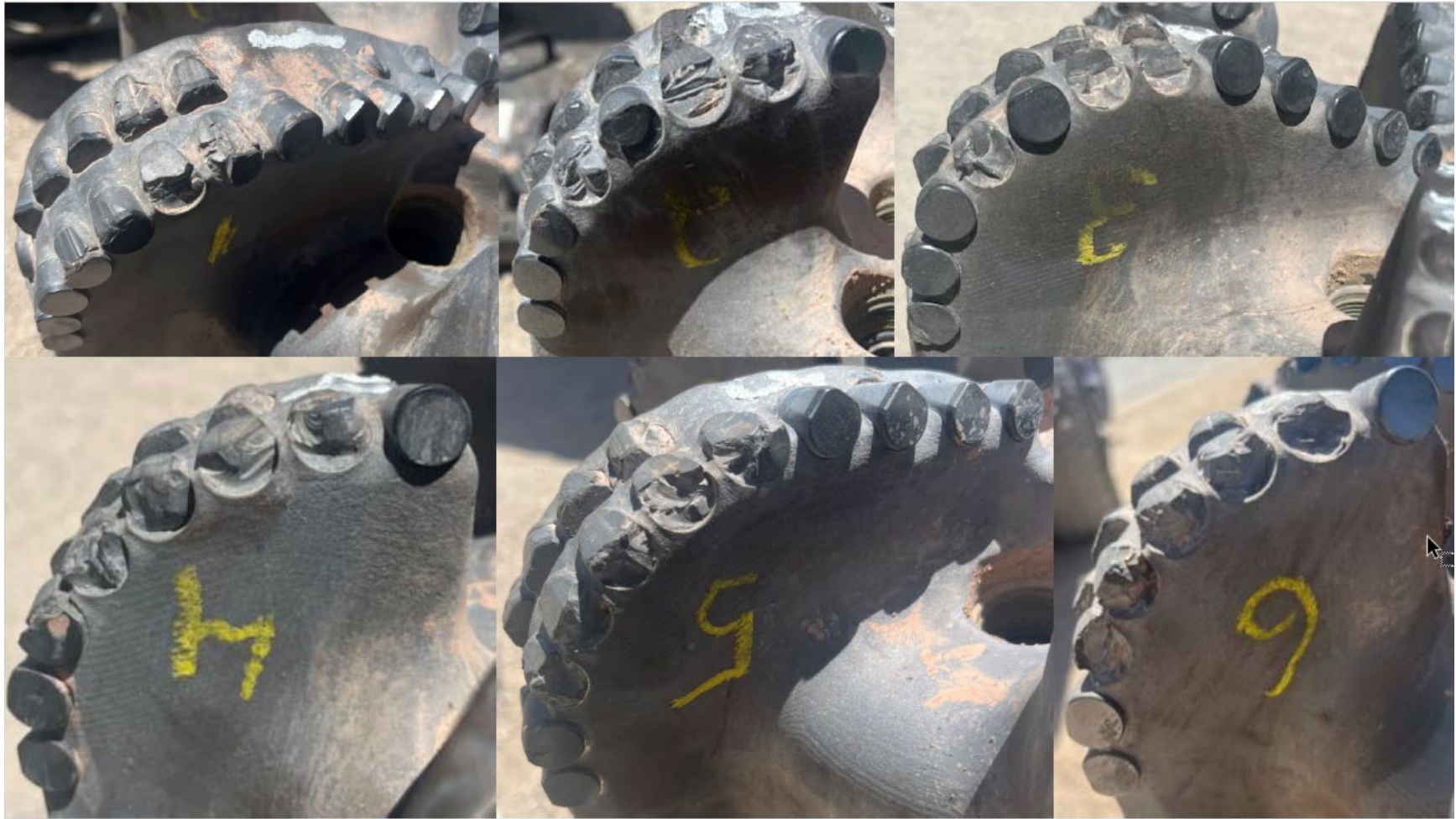
Figure 24. Post run dull photographs after pulling BHA#3. Note - ReedHycalog refers to this as BHA #2 - it is in fact BHA #3. This was an NOV TK66 PDC bit.
