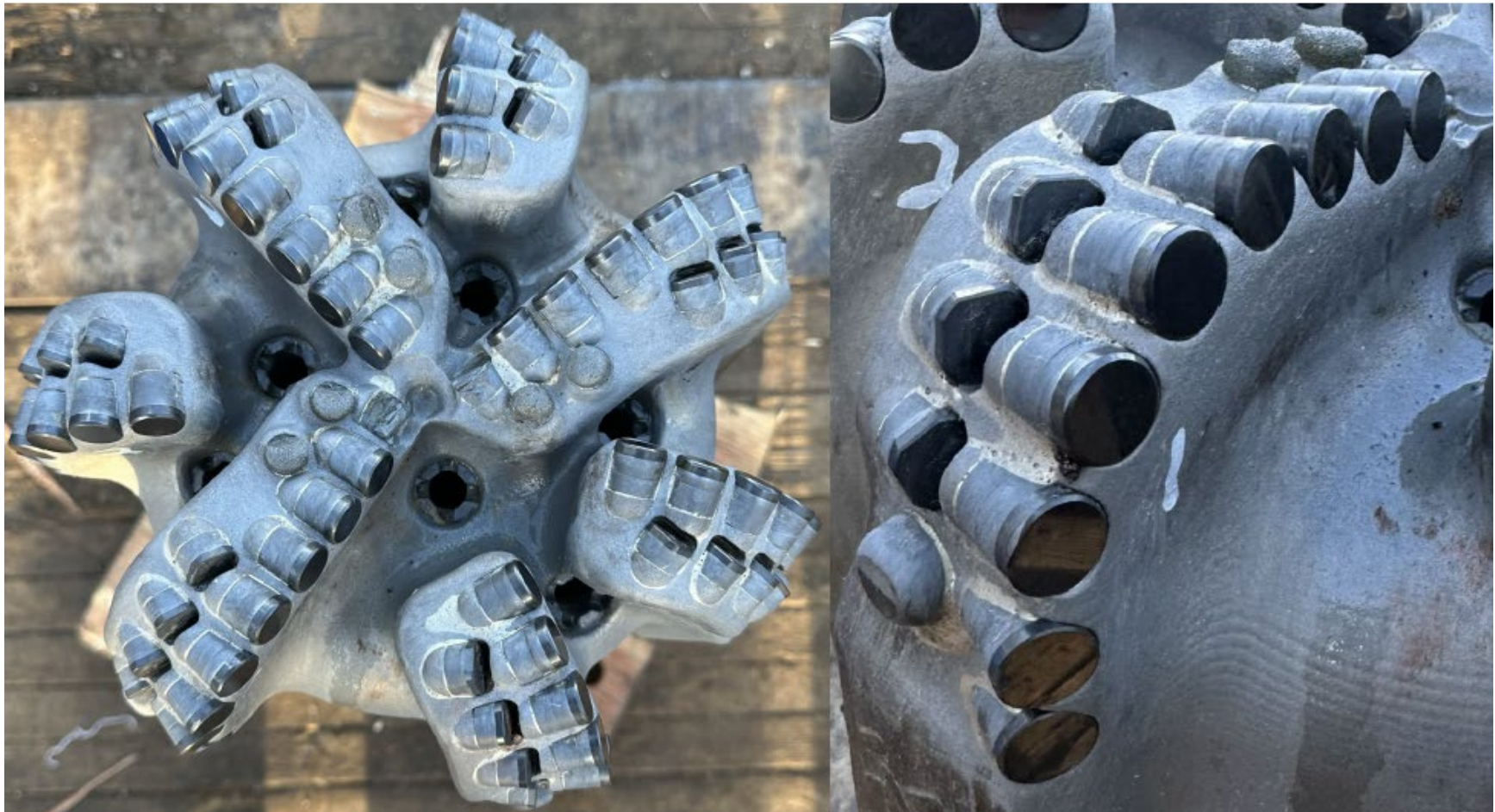
Figure 68. BHA #13 [9.5" TKC73-A2 (A298330)]. Compilation of dull photographs after drilling from 5,957 to 6,545 ft MD. Note - ReedHycalog and SDI refer to this as BHA #6 - it is in fact BHA #13. This was an NOV TKC73-A2 PDC bit.
