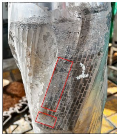
Figure F-3. Severe damage to the stabilizer and roller reamer.
