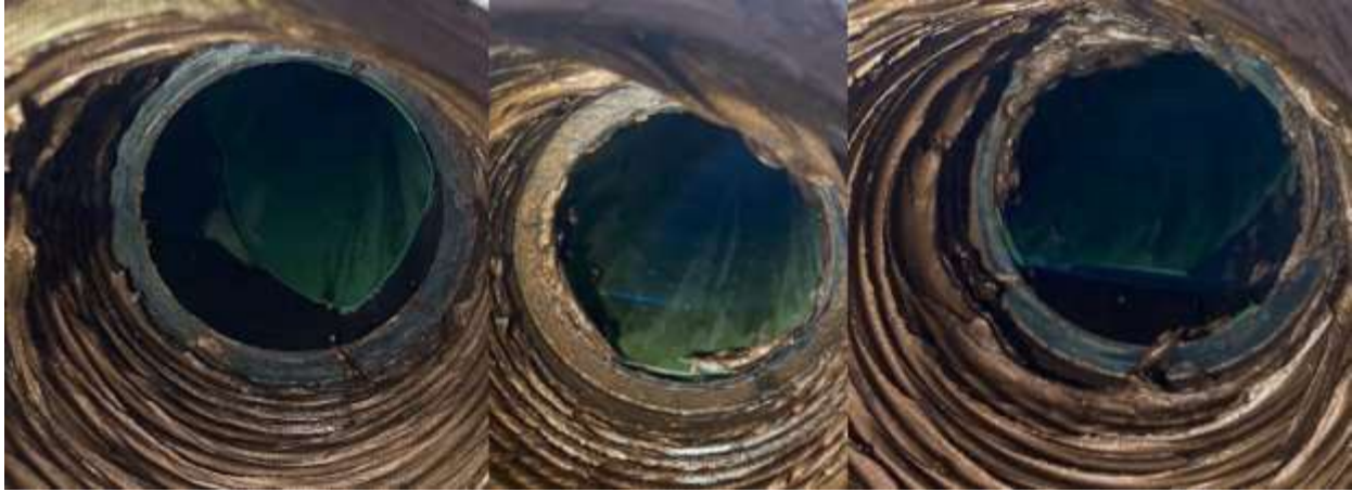
Figure D-8: Drill pipe joints laid down with ID coating defects
