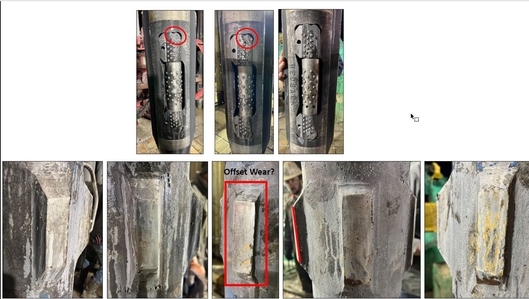
Figure F-61. There is some damage to the stabilizer and the roller reamer in this run.
