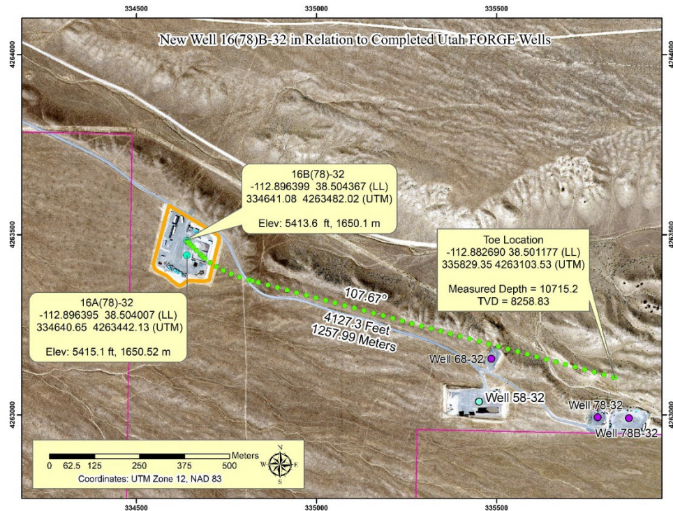
Figure 4. Plan view showing wellbore spud location for well 16B(78)-32, and its azimuth, drilling from west to east. North is to the top of this image. The location of 16A(78)-32 is also shown (spud and toe)
