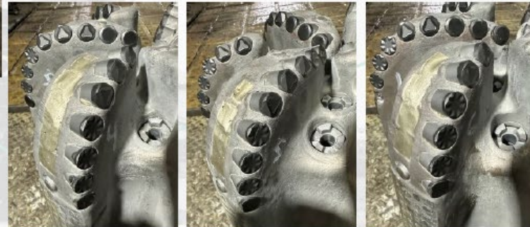
Cracked shoulder cutter
