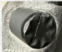
Cracked shoulder cutter
