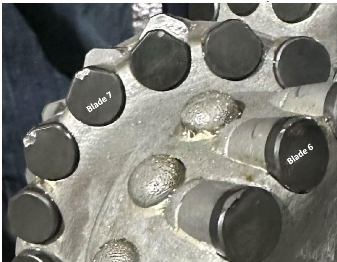
Figure 97. BHA #18 [9.5" TKC83-A2 (A298356)]. Dull photograph after drilling from 8,085 to 8,585 ft MD. Note - ReedHycalog and SDI refer to this as BHA #11 - it is in fact BHA #18. This was an NOV TKC83-A2 PDC bit. Pulled on schedule to test different bit performances.
