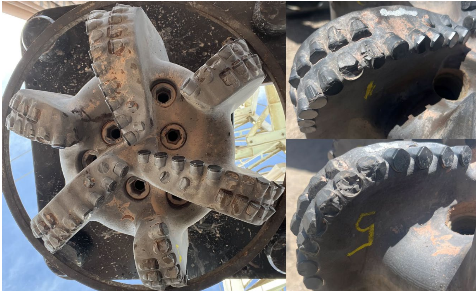
Figure 22. Post run dull photographs after pulling BHA#3. Note - ReedHycalog refers to this as BHA #2 - it is in fact BHA #3. This was an NOV TK66 PDC bit.
