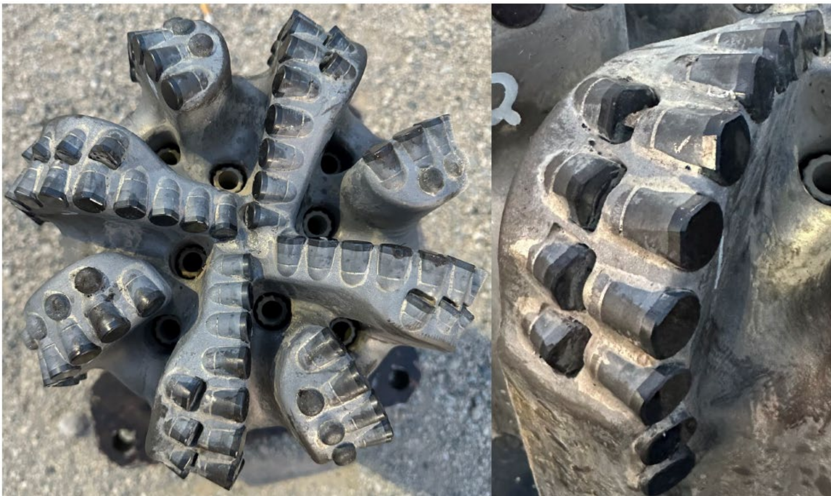
Figure 73. BHA #14 [9.5" TKC83-A2 (A298355)]. Compilation of dull photographs after drilling from 6,545 to 6,610 ft MD. Note - ReedHycalog and SDI refer to this as BHA #7 - it is in fact BHA #14. This was an NOV TKC83-A2 PDC bit. Pulsar on directional tool failed.
